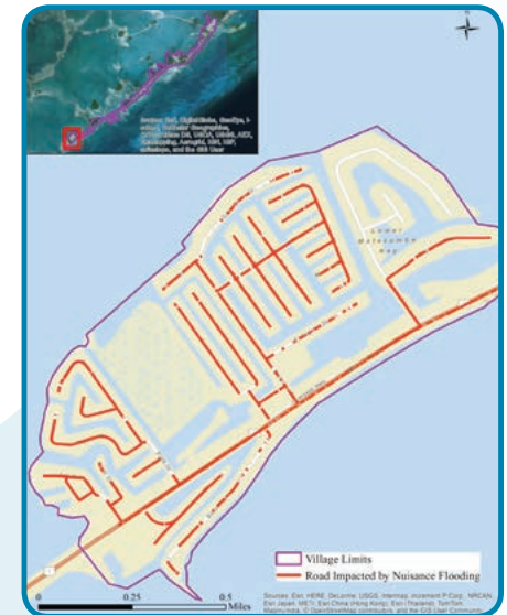
Figure 3: Road segments predicted as vulnerable to nuisance flooding with 24 inches of sea level rise (2060, High Scenario). (See Appendix B for larger image)
