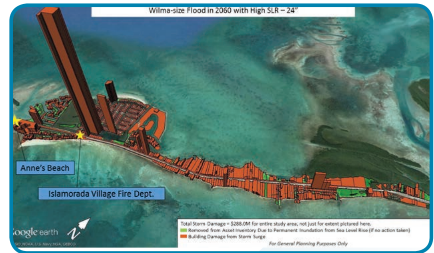
Figure 5. Google Earth image of potential flooding damages from a Hurricane Wilma-size flood (high sea level rise scenario) in 2060 for a section of Islamorada, FL. Coral parcels indicate those flooded from storm surge, with the height of the coral extrusions representing relative damage amounts (in dollars). Parcels in green indicate those permanently inundated from sea level rise. (See Appendix D for larger image)
